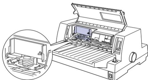
5. Turn the ribbon-tightening knob on the ribbon cartridge in the direction of the arrow to take up any slack in the ribbon.
