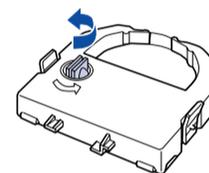
6. Hold the ribbon cartridge with the exposed ribbon down and the ribbon-tightening knob facing you, and guide the ribbon under the print head. Then snap the cartridge into place so that the tabs on both sides of the cartridge fit into the notches in the cartridge holder.
