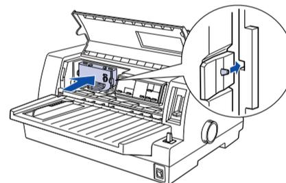
8. Turn the ribbon-tightening knob again to remove any slack in the ribbon and to make sure the ribbon moves freely.
