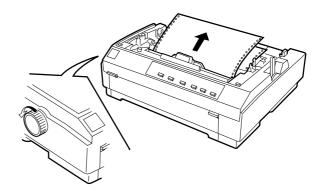
Turn the knob on the left side of the printer away from you to eject the paper in the printer. Remove any remaining pieces of paper.
