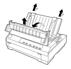
Remove the printer cover. If continuous paper is jammed in the rear slot, also remove the paper guide.
