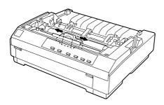
Slide the print head from side to side to make sure it moves smoothly. Also check that the ribbon is not twisted or creased.
