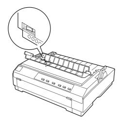
Turn off the printer. The power switch is located on the left side of the printer.
