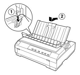
Attach the paper guide, then lift the center section of the paper guide up and lay it flat.
