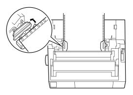
Open both sprocket covers, and fit the first three holes of the paper, printable side down, over the tractor pins. Then close the sprocket covers.
