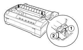
To replace the paper tension unit, lower it onto the printer's mounting pegs. Then press down both ends of the unit until it clicks into place.
