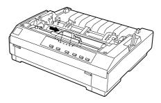
Make sure the print head is not hot; if it is, let it cool for a few minutes before touching it. Then slide the print head to the middle of the printer by hand.
