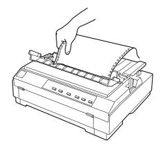
Open the paper path guide cover, and tear off the printed document using the printer's tear-off edge.
