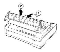
Open the paper guide cover. Then lift the printer cover by its back edge and pull it straight up and off.
