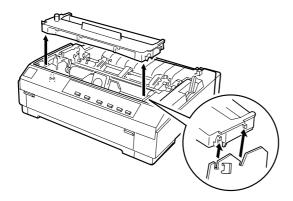
Grasp the cartridge by its handle and pull it straight up.
