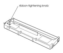
Take out a new ribbon cartridge. Turn the ribbon-tightening knob in the direction of the arrow to remove any slack in the ribbon.
