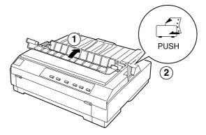
Close the paper guide cover, and make sure the paper release lever is set to the push tractor position.
