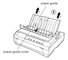
Turn off the printer, then open the paper guide cover and remove the paper guide.
