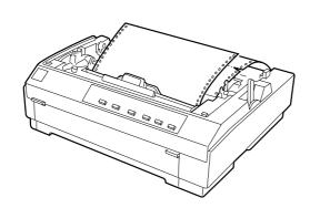
If continuous paper is jammed inside the printer, tear off the supply at the perforation nearest the paper entry slot. **5**
