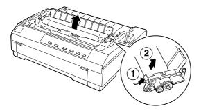
Push up the tabs on each side of the paper tension unit and lift the unit up and off the printer. Store the paper tension unit in a safe place. When the pull tractor is installed, it is not necessary to remove the paper tension unit.
