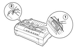
Use a pointed object, such as a ball point pen, to guide the ribbon between the print head and ribbon guide. Turn the ribbon-tightening knob to help feed the ribbon into place.
