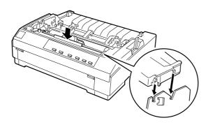
Hold the ribbon cartridge by its handle and push it firmly down into position. Then press on both ends of the cartridge to make sure the plastic hooks fit into the slots.
