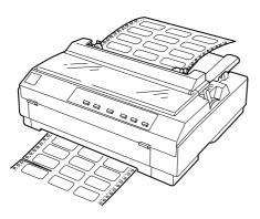
Tear off the supply of continuous labels at the perforation nearest the paper entry slot.
