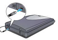
5 Connect the power cord and the AC adapter, and then connect the power cord to the scanner.
