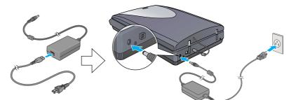
The scanner turns on and the & Start button light flashes in green. It stops flashing and turns green when the scanner is ready.
