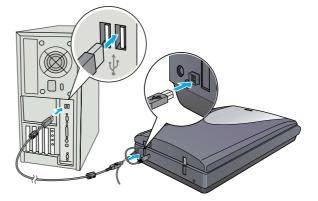
Caution: The interface cable connectors have only one correct orientation. Ensure the correct orientation of a connector before inserting it into the appropriate port.
