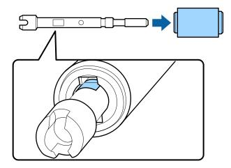
Attach the new middle pickup roller to the axis.
