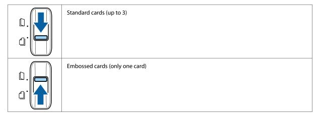
Load the card into the input tray with the printed side facing down and the top edge facing into the feeder. Slide the card into the feeder until it meets resistance. Then slide the edge guides to fit the edge of the card.
