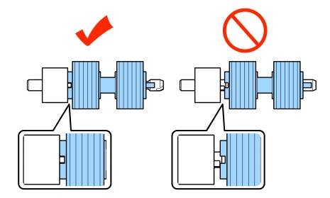
Attach the new separation roller to the correct position. Make sure the notches align.
