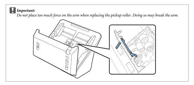
5 Slide and remove the installed pickup rollers.
