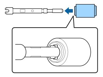
Remove the lower pickup roller from the axis.
