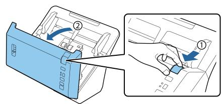
Press the hook on the right side of the pickup roller cover, and then open the cover.
