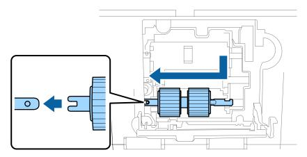
Attach the new middle pickup roller in the correct position.
