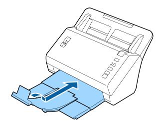
Remove the input tray by pulling it towards the scanner cover.
