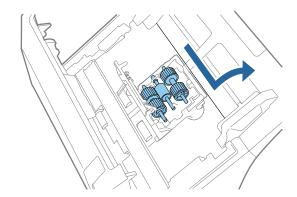
Remove the upper pickup roller from the axis.
