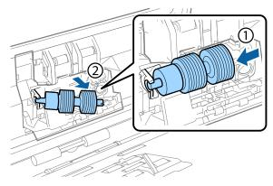
Remove the roller from the axis.
