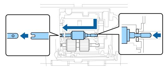
11 Attach the new upper pickup roller in the correct position.
