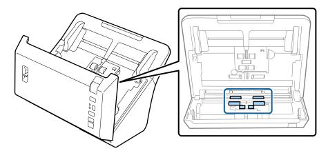
Wipe off any stains on the pickup roller.
