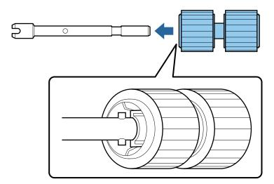
Attach the new lower pickup roller in the correct position.
