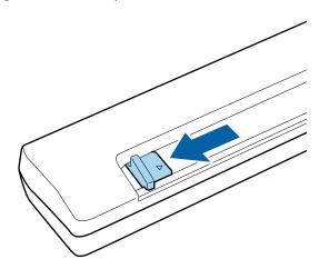
2 Load your document with the printed side face down and the document edge aligned with the right edge of the input slot until the top edge of the document is gripped by the product. If the product does not grip the document, try loading it again.
