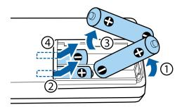
Insert the batteries matching the positive and negative terminals of the batteries and the marks inside the battery compartment.
