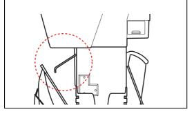
5 For Epson Stylus Pro 9900/9910, switch the position of the rear paper basket depending on the paper size.
