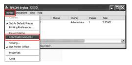
If the job has been sent to the printer, the print data does not appear in the dialog box above. In this case, cancel the print job using the printer.
