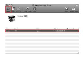
If the job has been sent to the printer, the print data does not appear in the dialog above. In this case, cancel the print job using the printer.
