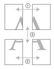
1 Cut the upper left sheet along the alignment mark (vertical blue line).
