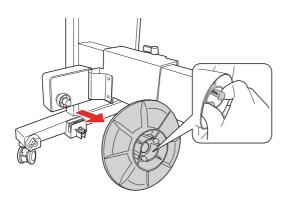
4 Reverse the flange so that the smaller knob is positioned on the outside, then replace it on the movable unit by pinching the knob.
