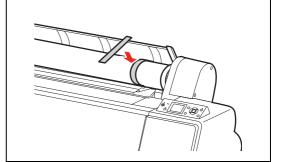
4 To unlock the adapter holder, push the lock lever of the adapter holder down firmly. Move the adapter holder to the left with the handle until the end. Then take it off from the holder axis.
