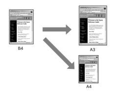
Fit to Roll Paper Width (Windows only) Proportionally enlarges or reduces the size of your data to make it fit the width of the roll paper you have selected in Output Paper list.
