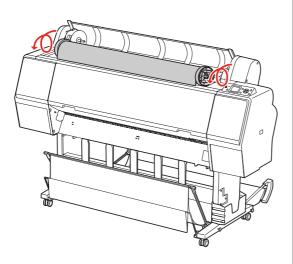
6 Pull up the lock lever of the adapter to unlock. Then remove the roll media adapter from the paper roll.
