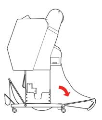
Tilt the front basket until parallel to the floor when ejecting your prints.
