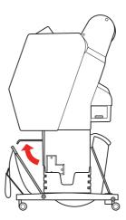
3 Remove the hook-and-loop fastener straps, and refasten it downward. Then bring the front paper basket up to the vertical position.
