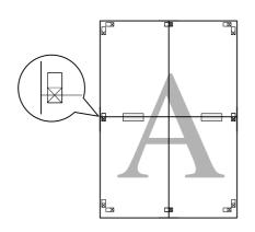
8 Cut the sheets along the alignment mark (horizontal red line).
