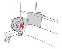
4 Turn the lock lever to the front to lock the movable unit.
