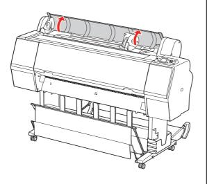
3 To unlock the adapter holder, push the lock lever of the adapter holder down firmly. Then move the adapter holder to the left with the handle.
