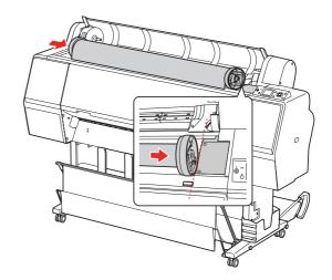
9 Slide the adapter holder with the handle to make the left roll media adapter align with ▲ on the adapter holder.
