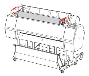
11 Slide the adapter holder with the handle to the right to set it in the holder axis firmly.
