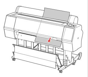
6 Make sure that the right and bottom edges of the sheet are straight and in line with the set line.
