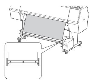
Press the  $\checkmark$  button to feed the paper forward and create a loop of slack.
