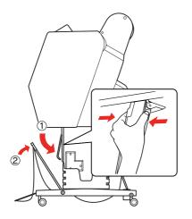
4 Bring the front paper basket up and fasten it with the hook-and-loop fastener straps.
