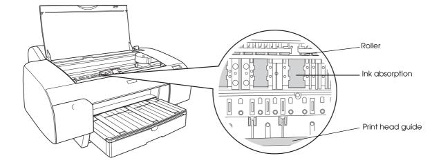
2. Open the top cover and then use a soft, clean cloth to carefully remove any dust or dirt inside the printer. Wipe the gray part by following the directions of the arrows.
