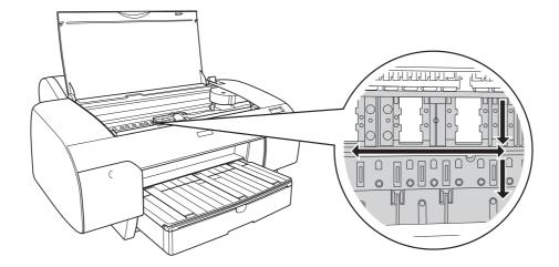
3. If the back of a printout is soiled, carefully clean the platen (the gray part) using a soft, clean cloth.
