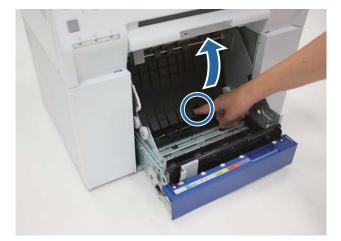
8 Check that there is no paper or foreign material at the back of the inside of the printer.
