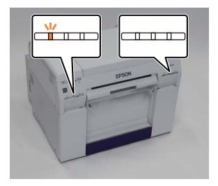
Open the cartridge cover on the side that needs to be replaced.
