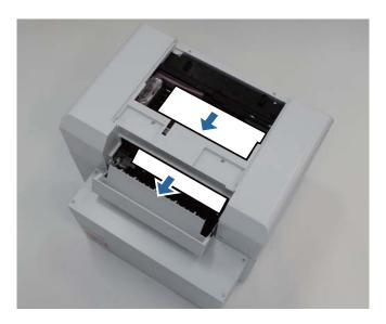
7 Move the Print head unit manually, and remove the paper from the rear.
