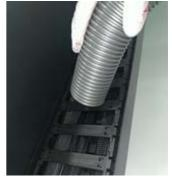
Use a vacuum cleaner and so on to suck up any dust that has accumulated on the filter for the UV lamp cooling unit.
