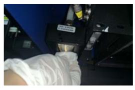
Do not touch the UV lamp during printing. It can become extremely hot and could cause injuries or burns. When performing maintenance, allow the lamp to cool for at least six minutes before you start.
