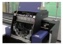
6-2 Use the wrench for sub ink tanks to close the valves in all of the sub ink tanks.
