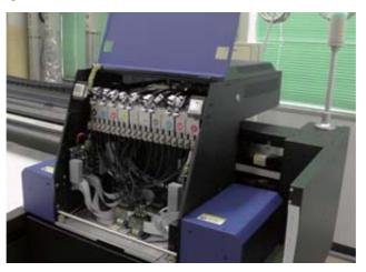
Use the wrench for sub ink tanks to open the valves in all of the sub ink tanks.
