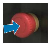
To release the emergency stop, turn the button clockwise.
