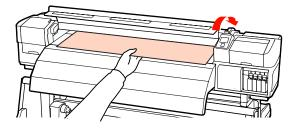
Pull the media straight forward until the edge has past the label on the left side of the after heater.
