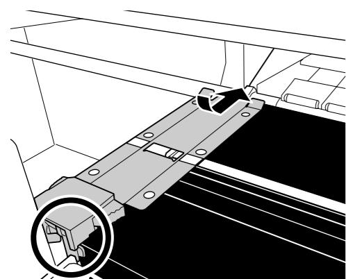
In the position where the white lines on the platen and the media holding plate make a straight line, press the tip of the metallic plate against the platen and attach the hooked sections.
