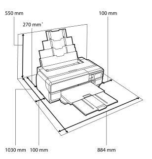
\* When printing on poster board, leave a space of at least 430 mm in behind the printer.
