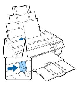
When the paper is loaded correctly, the Paper Setup screen is displayed.
