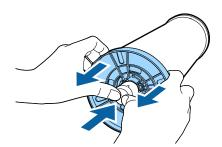
If it is difficult to remove, tap gently on the tip of the spindle on the black flange side.
