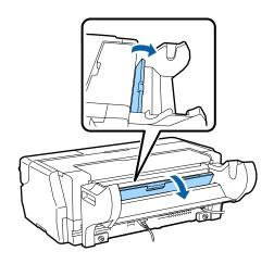
Load the spindle with the roll paper into the unit.
