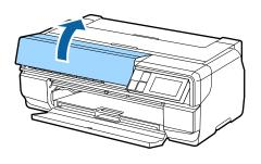
*Important:* Do not force open the ink cartridge cover until the lock is released.
