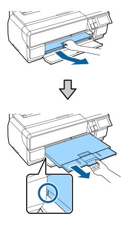
When the paper is loaded correctly, the Paper Setup screen is displayed.
