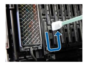
(3) Flatten the cleaning stick and wipe all of the edges of the drying caps.
