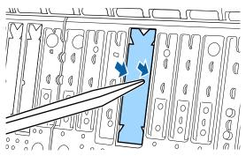
Gently press the pad for borderless printing until it is seated flatly in place.
