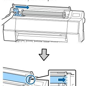
Raise the lock levers on the adapter holders to lock them in place.
