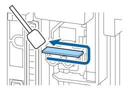
(3) Wipe any dirt off the upper edge of the wiper (three parts).
