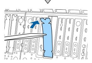
Press the pad for borderless printing into the pad section.
