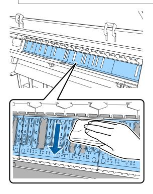
If any paper particles (resemble white powder) have accumulated in the holes shown in the illustration below, use a pointed object such as a toothpick to push them in.
