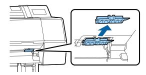
Loosen the screw that secures the cutter with a cross-head screwdriver.
