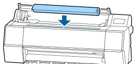
Adjust the size of the roll paper adapters to the size of the roll core.
