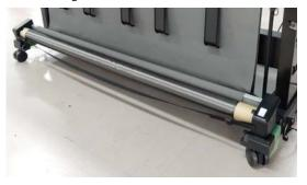
Remove the optional auto take-up reel unit or SpectroProofer mounter if they are installed.
