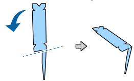
Insert the leg of the pad for borderless printing all the way into the hole.
