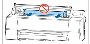
Raise the adapter lock levers to release the locks, and remove the roll paper adapters from the roll paper.
