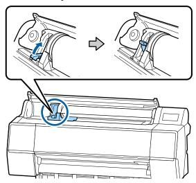
Insert the leading edge of the roll paper into the paper feed slot, and continue to feed until you hear a sound.
