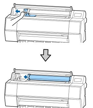
Roll over the paper roll to the front side to place it on the top of the printer.
