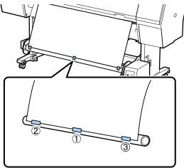
Flip the Manual switch on the auto take-up reel unit to Forward, and take up as much paper as possible.
