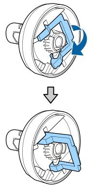
Attach the roll paper adapters to both ends of the roll paper, and then lower the lock levers on the left and right to lock them in place.
