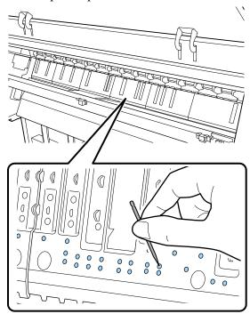
Remove paper particles and dust around the outer edges with commercially available cotton swabs as shown below.
