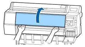
Clean the platen near the back where soiling occurs.
