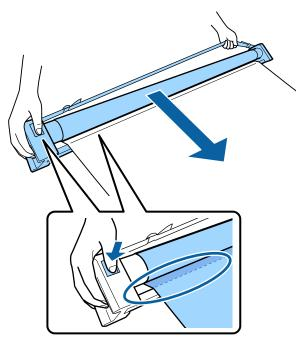
Place the roll in the position shown in the illustration of the stand.
