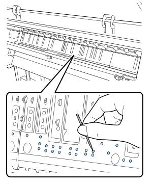
Use a commercially available cotton swab to wipe off the paper particles and dust from the inner edges of the pads for borderless printing as shown below.
