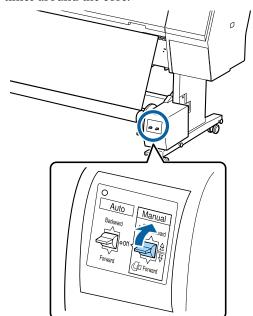
After wrapping the paper around the core, ensure that paper around the core is sufficiently loose.
