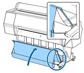
When the cloth touches the floor, secure using the hook and loop fastener tape as shown in the illustration.
