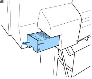
Place the used maintenance box in the clear bag included with your new maintenance box, and make sure that the zipper is closed tight.
