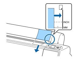
For paper smaller than A4 size, insert by keeping the right edge aligned with the additional line below the paper feed slot.
