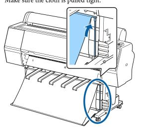
4 Lower the paper supports while pressing left and right as shown in the illustration until they touch the cloth.
