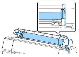
14 Raise the lock levers on the adapter holders to lock them in place.
