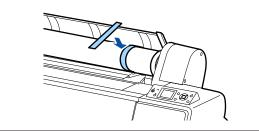
4 Lower the lock lever for the adapter holder to release the lock.
