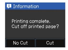
**Cut**: Feeds roll paper to the cutting position.
