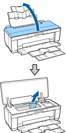
After removing the paper, close the printer cover and press the Ph button to cancel the error.
