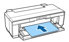
Match the edge guide to the width of the paper and align the trailing edge with the triangles at the left and right sides of the tray.
