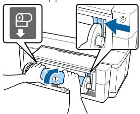
Slide the roll paper in until it stops and keep it lightly held in this position for about three seconds.
