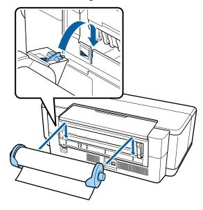
6 Lightly insert the roll paper into the rear roll paper feeder and match the edge guide to the width of the paper.
