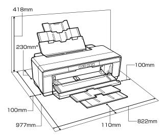
\* When printing on thick paper, leave a space of at least 320 mm behind the printer.
