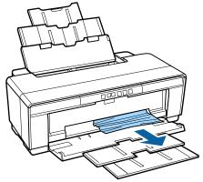
Open the printer cover and slowly pull the jammed paper out of the printer.
