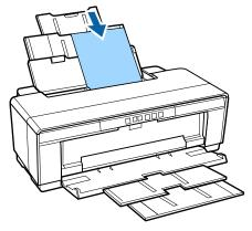
Grasp and slide the edge guide to fit it to the width of the paper.
