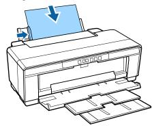
Slide the paper in until it stops and keep it lightly held in this position for about three seconds.
