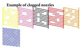
If any segments are missing in the nozzle check pattern, perform head cleaning.
