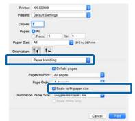
Select the size of the paper loaded in the printer as the **Destination Paper Size**.
