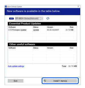
When Firmware Updater is displayed, the latest firmware is available. Select Firmware Updater and click the Install button to automatically start Firmware Updater and update the printer firmware.
