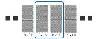
If all of the adjustment patterns contain overlapping or gaps, select the pattern with the least overlaps or gaps. Perform steps 2 to 4 again, and repeat them until a pattern with no overlapping lines or gaps is printed.
