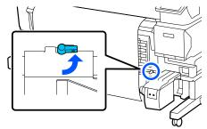
Align the right-side roll core holder with the edge of the media.
