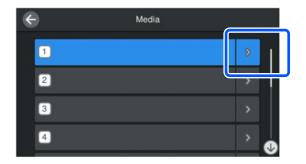
Select the Media Type using the paper weight of the loaded media as a guideline as shown below. The paper weights of each Media Type shown on the screen are typical values.
