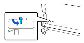
Check the winding direction, and then in the order shown in the illustration below, use commercially available tape to stick the media to the roll core. When attaching in the center, attach using tape while pulling the center of the media straight. When attaching to the left and right sides, attach using tape while pulling the media to the side.
