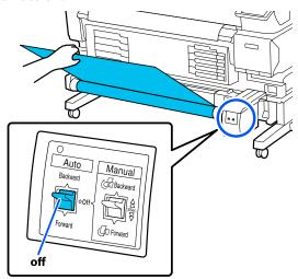
Set the Manual switch so that it matches the winding direction, and then wind the cut media.
