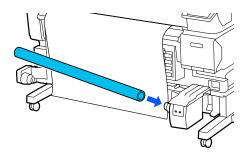
Make sure the roll core holder is inserted into the roll core and that the roll core and the edges of the media are aligned.
