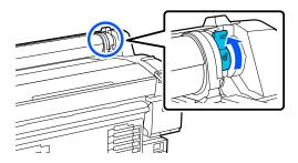
Holding the roll adapters on both sides, move the media to the roll rest.
