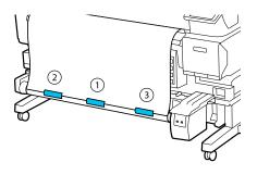
Press the button until you have fed enough media for about one full wrap around the roll core.
