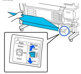
Unlock the lock lever on the left-side roll core holder, and then remove the roll core holder from the roll core.
