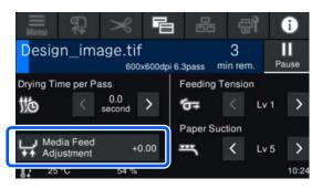
If the home screen (adjust while printing) is not displayed, press 旨 (switch screens) on the home screen.
