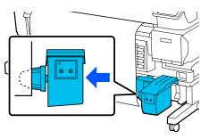
Move the lock lever on the roll core holder to the lock position to secure the roll core holder.
