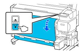
Set the Manual switch so that it matches the winding direction, and then wind the media once around the roll core.
