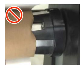
□ Depending on the media type and media width, the media may become misaligned with the roll or too loose and then cause an Auto Take-up Reel Unit Error when taking up over a long distance.
