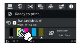
Operation areas do operations when pressed. However, when a scroll bar is displayed as shown below, you can scroll the screen by moving (sliding) your finger up and down on the screen. You can also scroll by pressing on the up and down icons on the scroll bar.
