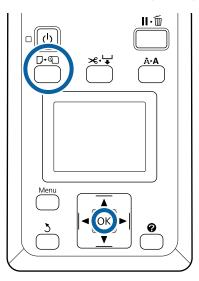
1 Check that **Press and load paper.** is displayed on the screen, and then open the roll paper cover.
