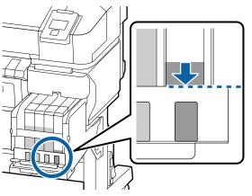
Make sure the ink level is below the top edge of the metal plate.
