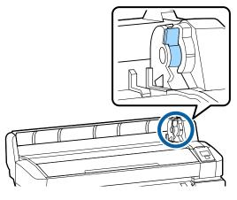
3 Slide the roll paper right until it contacts the adapter guide. Next, following the adapter guide, slide the roll slowly inside.
