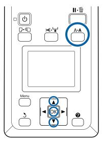
1 Confirm that the printer is ready to print. Press the A>A button.
