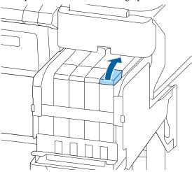
Remove the ink inlet cap from the ink tank. The method for removing the ink inlet cap differs depending on the type of ink being refilled.
