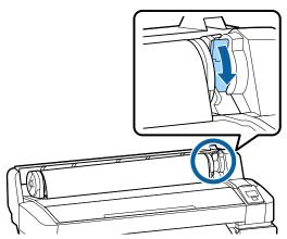
If the leading edge of the paper is not horizontal or not cut neatly, you can cut the edge of the roll paper with the built-in cutter by pressing the OK button, and then pressing the ≫.↓ button within five seconds.
