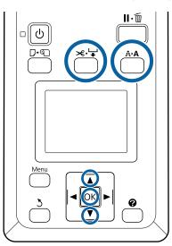
Confirm that the printer is ready to print. Press the A>A button.
