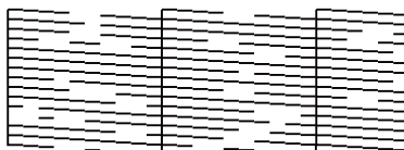
Example of clogged nozzles
