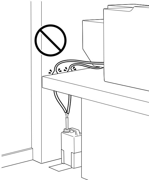
Do not bend or pinch the waste ink tube. This could cause ink to leak inside or around the printer.
