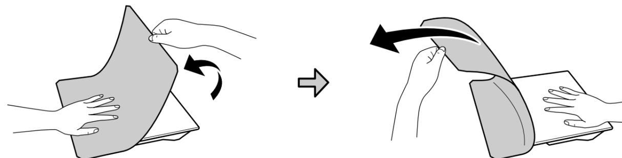
Do not use a dryer when removing the pad, as the heat could warp the platen. Use a commercially-available spatula if the pad is difficult to remove. Any remaining adhesive can be removed with a neutral detergent.
