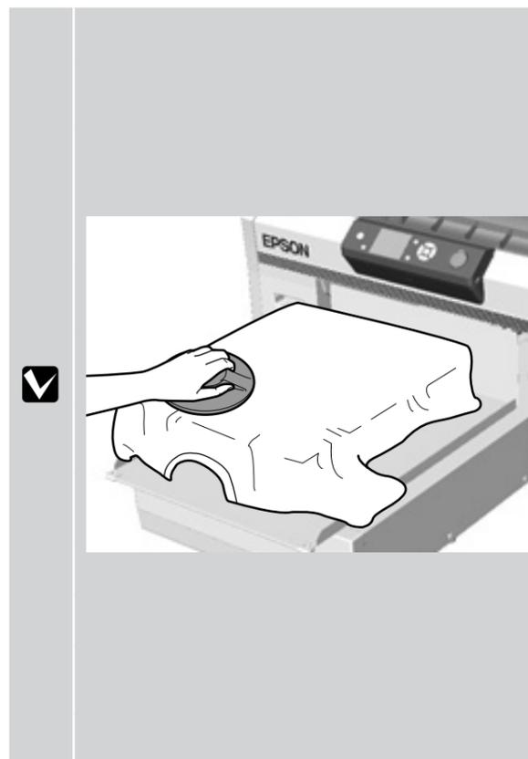
Use the Grip Pad Tool (a disk-shaped press, option) to flatten the print surface after loading the media.
