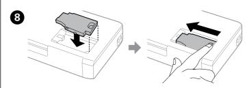
Place the new maintenance box straight down, and then slide it to install
