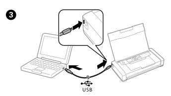
Connect the printer to the computer using a micro USB cable.
