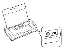
Turn on when the power is on. Flashes when the error occurs.
