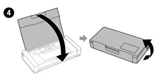
Close the printer cover, and then turn the printer over.
