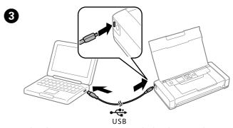
When the on-screen instructions are displayed, connect the printer and the computer with a micro USB cable, and then press the **OK** button on the control panel.
