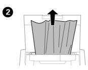
If the jammed paper remains inside the rear paper feed, carefully remove the paper.
