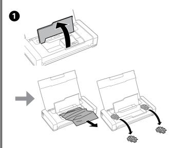
Open the inner cover and remove the jammed paper.
